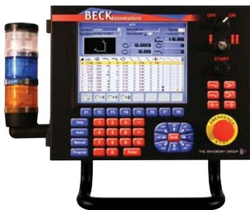
Bradbury folders come with the Beck Automation Intelli-Fold™ Controller featuring selectable bend allowance, material thickness adjustment, and compact flash memory for easy data back up and transfer. The controller is preloaded with a library of standard trim parts, has touchscreen editing to create new parts, and a graphic display that illustrates how to position the blank while forming the part.
